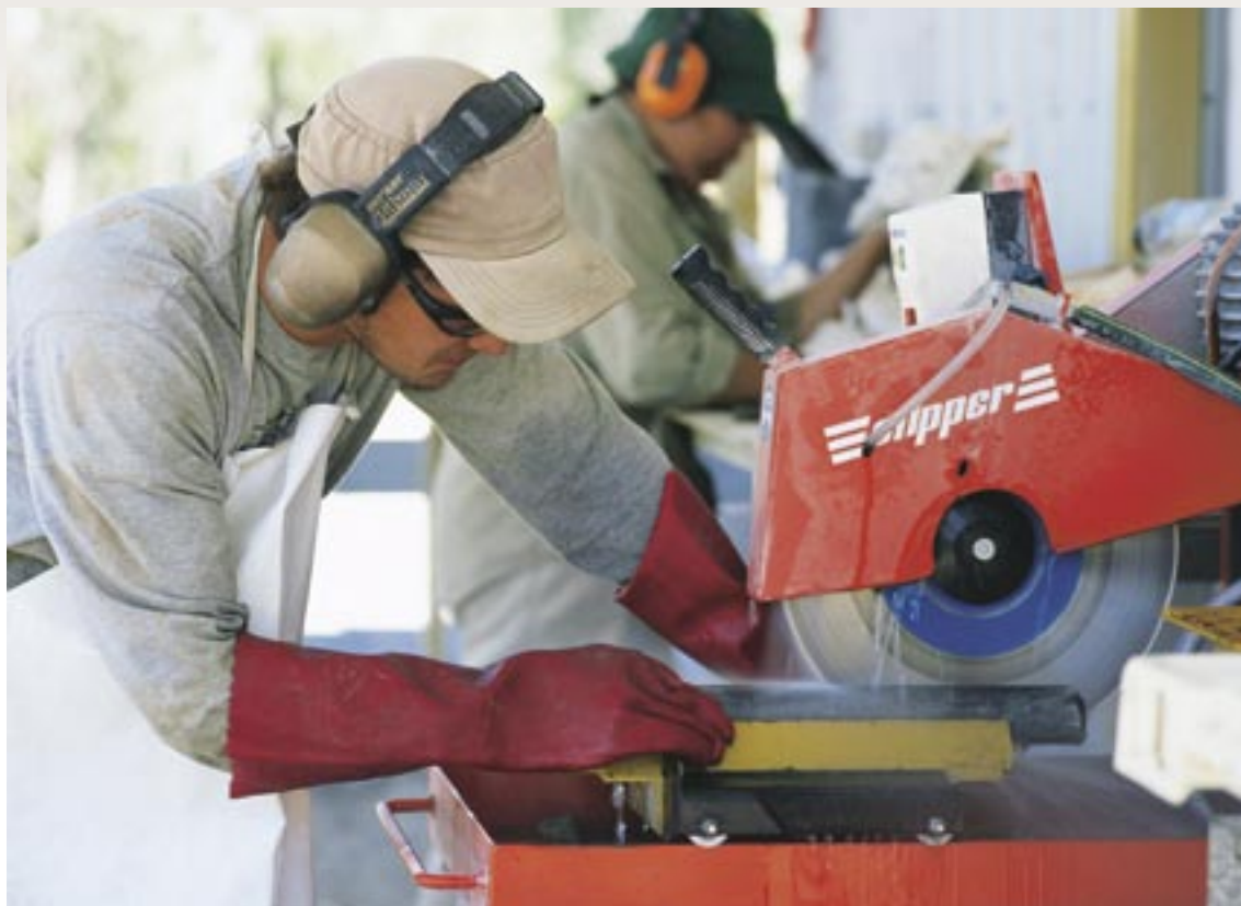
Cutting core at Watershed.
