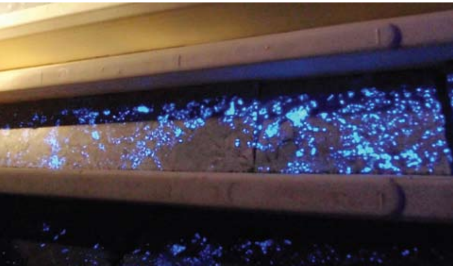
Scheelite in Watershed drill core (fluorescing under ultraviolet light).
