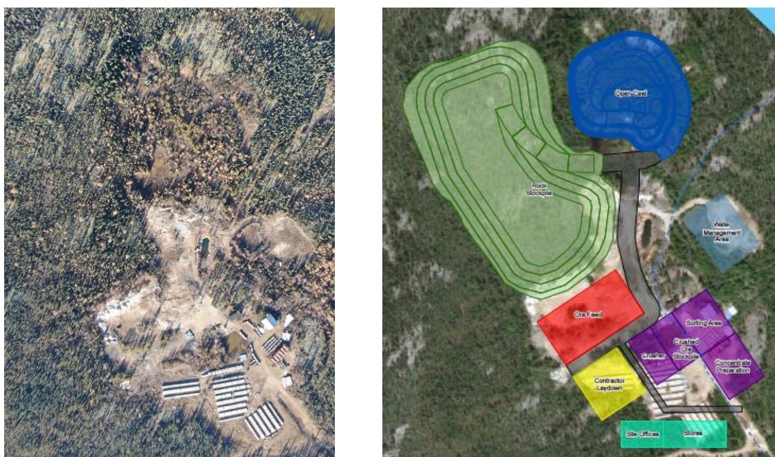
Figure 1: Approved site layout at North T Zone showing rock stockpile, ore feed, open cast pit and infrastructure
