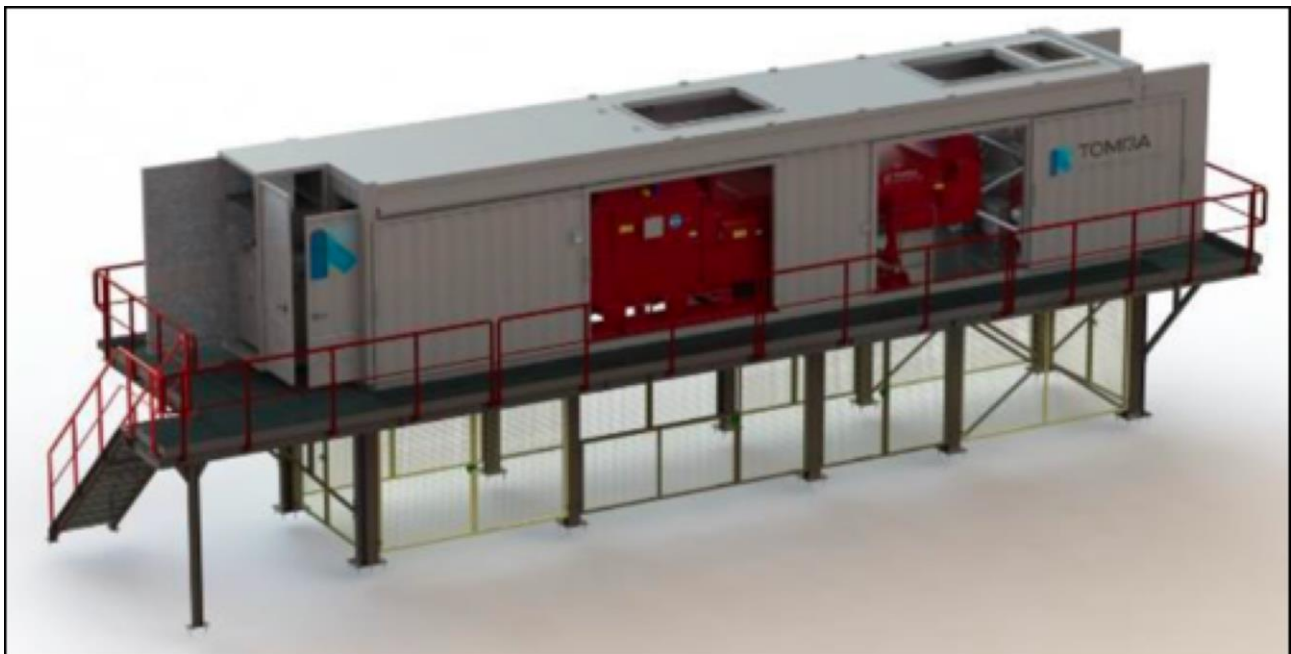
Figure 8: Schematic of Ore Sorter, in place with support structure.
