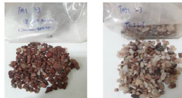
Concentrate sample via gravity
