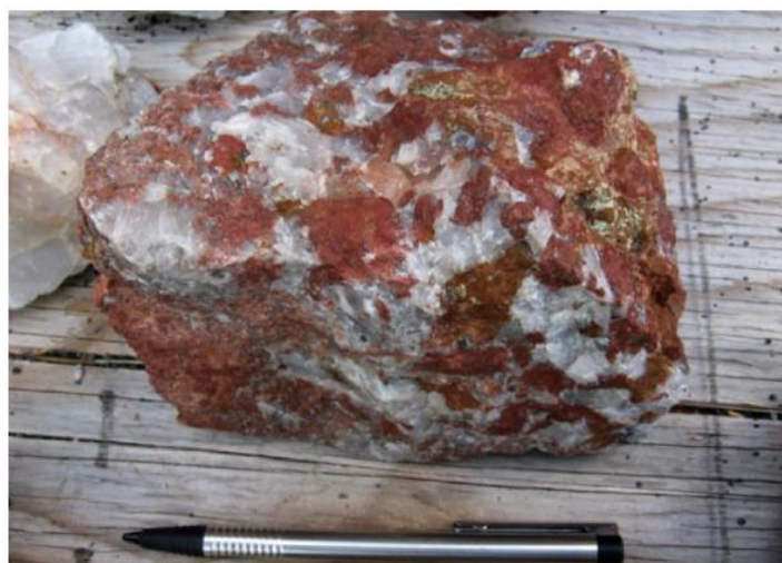
Figure 15: Ore sample from North T Zone showing red bastnaesite crystals (RE mineralisation) with quartz gangue
