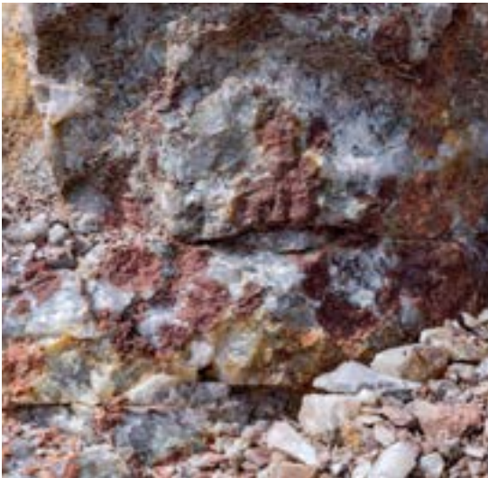
Large red nodes of high grade bastnaesite make it ideal to produce concentrate with sorter technology.
