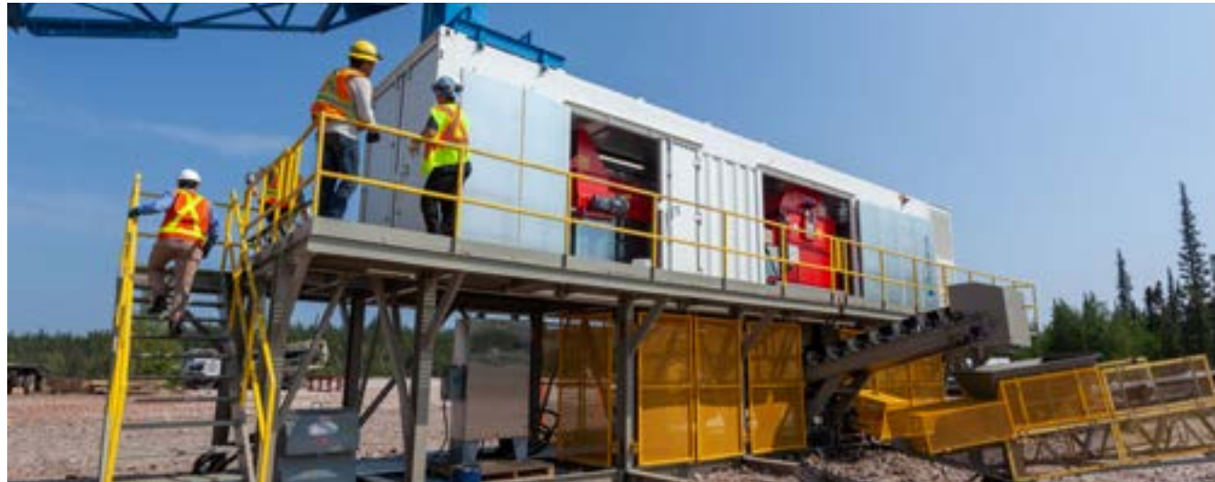
The TOMRA sensor-based sorter is a self-contained, portable machine that processes REE ore without water or chemicals, leaves no tailings and has a much smaller carbon and site footprint than conventional mining.
