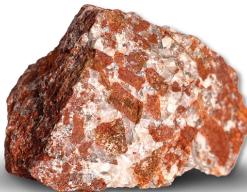
The brown REE mineral bastnaesite is mined and separated from the white quartz matrix into a mineral concentrate at Nechalacho mine.
