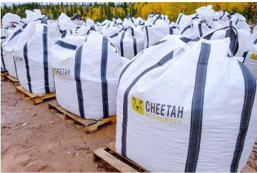
PhotoCaption: The mineral enriched by the sensor-based sorter is crammed into large bags that will take the road to Saskatoon. (Photo credit: Marie-Soleil Desautels)
